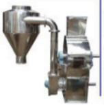
We offer Micro Pulveriser for Powdering / Grinding the dry materials like Chilly Powder, Spice powders, herbal leaves, animal feed materials, De oiled cakes, Husks, Ragi Powder etc.
