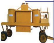
This machine is used to cook the raw turmeric by steam. And it is mobile type, can move one place to other place very easily.
