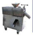
Double screw juice expeller is used for continuous extraction of juice from leaves, roots, stem, coconut and fruits.
